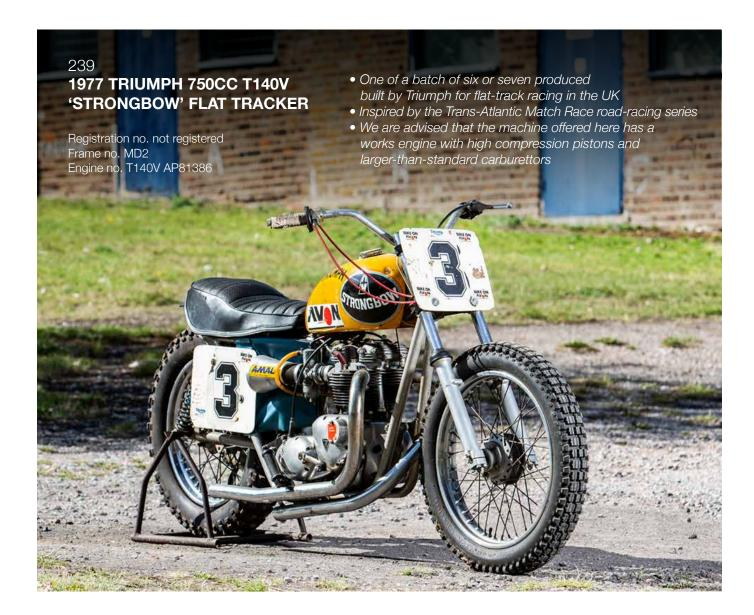
The machine offered here is one of a batch of six or seven (sources vary) T140V Bonnevilles built by Triumph for flat-track racing in the UK towards the end of 1977. Cider maker Bulmers was involved in sponsoring grass-track racing to promote its Strongbow brand, and commissioned Triumph to build these special Bonnevilles, the idea being to establish a 750cc class for solo machines. The transformation involved reverting to a right-side gearchange, standard up to 1975.
