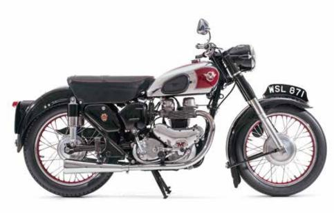
Announced in 1948, the Matchless G9 and equivalent AJS Model 20, while following the established pattern of British parallel twins, were unusual in having a third, central, crankshaft main bearing.
