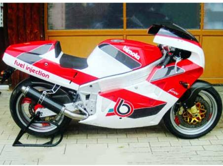
"The Furano, meanwhile, is Bimota's ultimate expression of the conventional hard-core take-no-prisoners sportbike, complete with low-mount clip-ons, adjustable suspension, carbon-fibre everything, modular wheels and an electronic engine management system." – Cycle World, July 1992.
